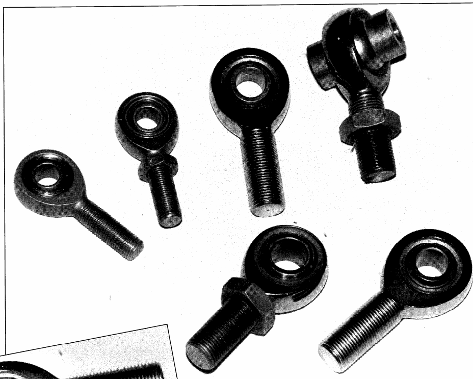
When shopping for rod ends, look for models like this three-piece precision design. The race is formed around the ball, then the race insert is staked into the body. This type of construction offers a much closer fit and a much higher degree of precision between the ball and the race. The three-piece design allows different materials to be used during construction, which makes for an ideal match of
